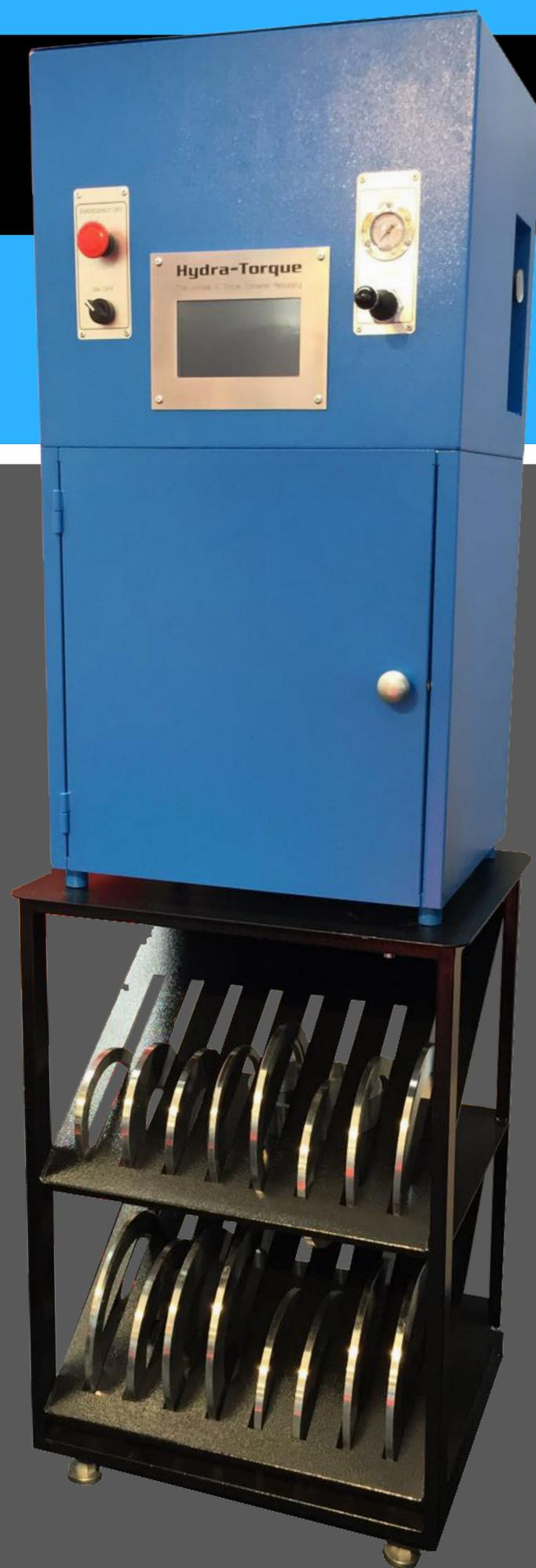
The Hydra-Torque piston bonder comes with a set of adapter plates covering an extensive range of transmission models.
